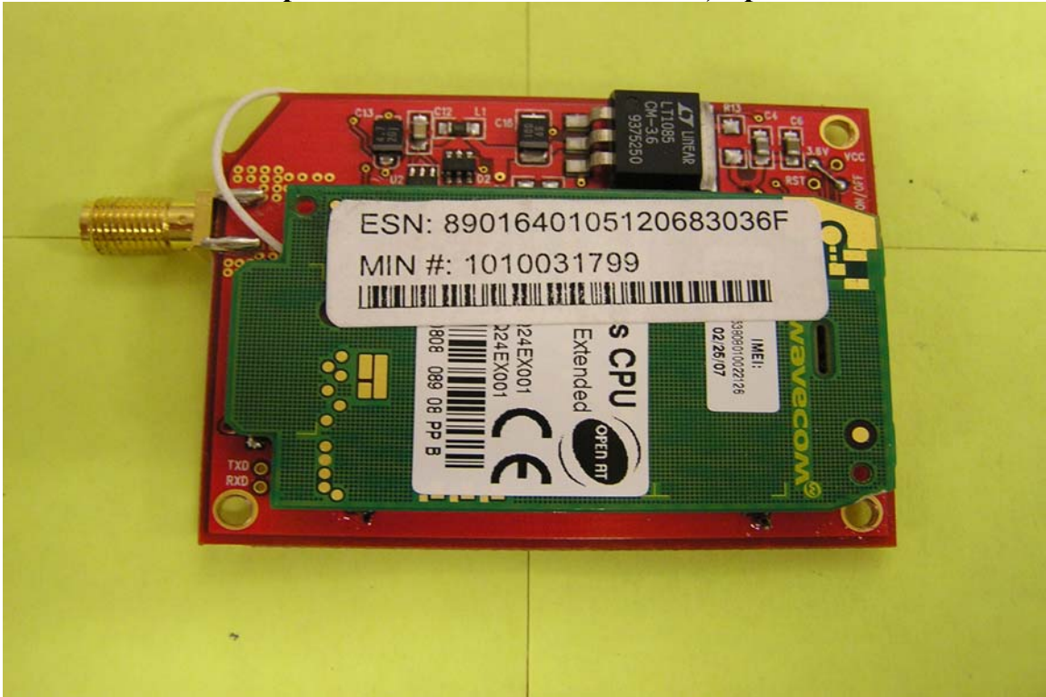
Prophet 4000 Picture 3: GSM module, top side
