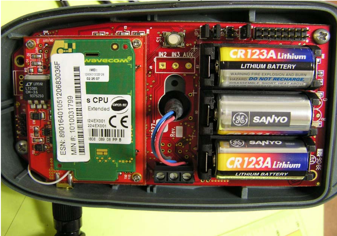
Prophet 4000 Picture 1: Internal photo, Front side PCB Board
