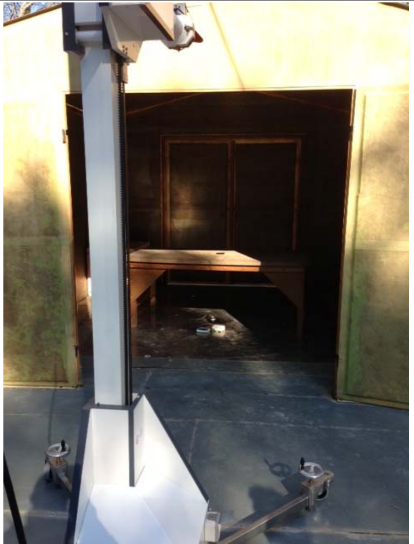
Open area test site measurement
