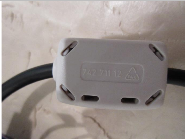
Ferrite bead Wurth Elektronik 742 711 12 was added to the 125 kHz antenna cable.
