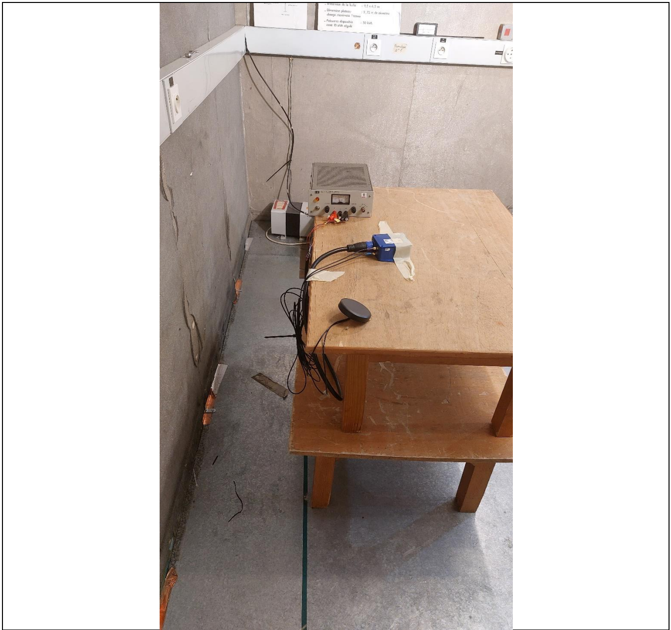
Test set up of conducted emission on power supply
