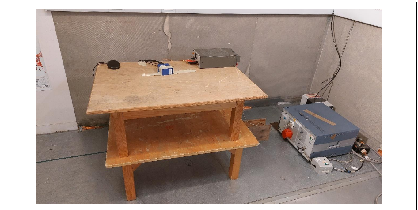
Test set up of conducted emission on power supply
