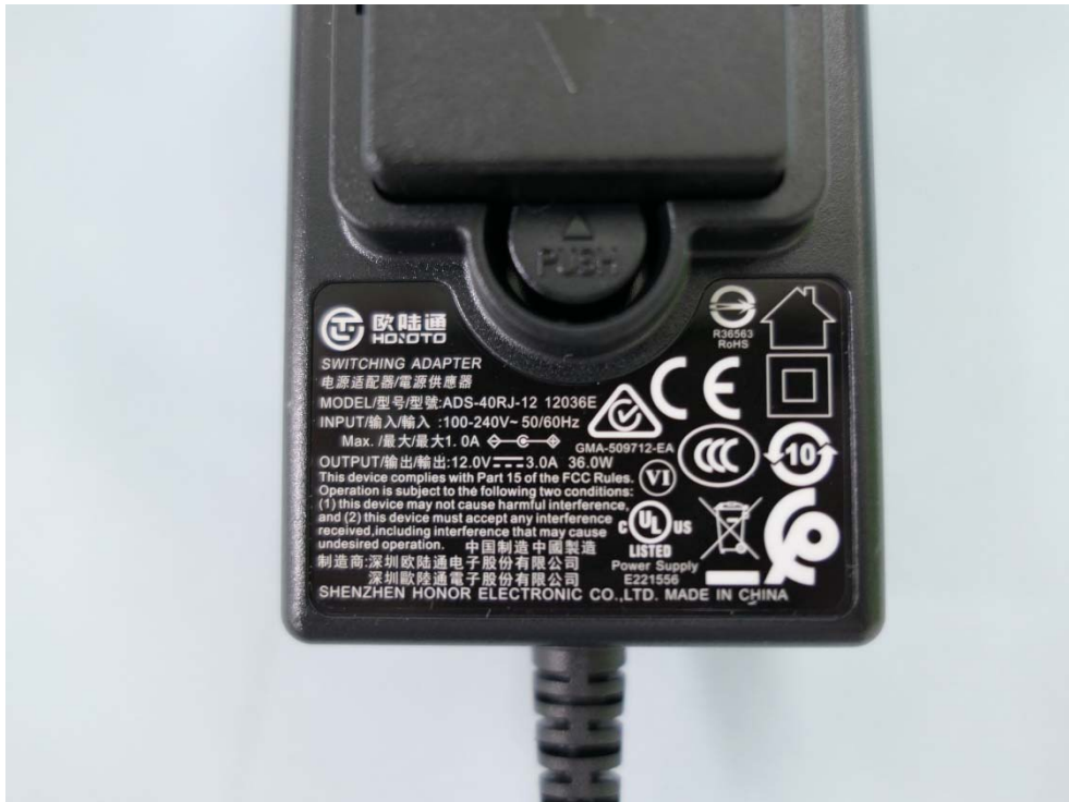
(14) Adapter (Brand: HOIOTO, M/N: ADS-40RJ-12 12036E)
