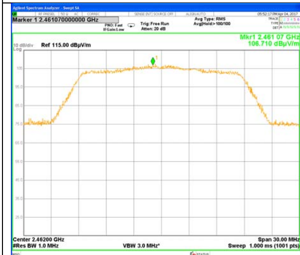
Plot # 21. Carrier frequency – 2462 MHz
