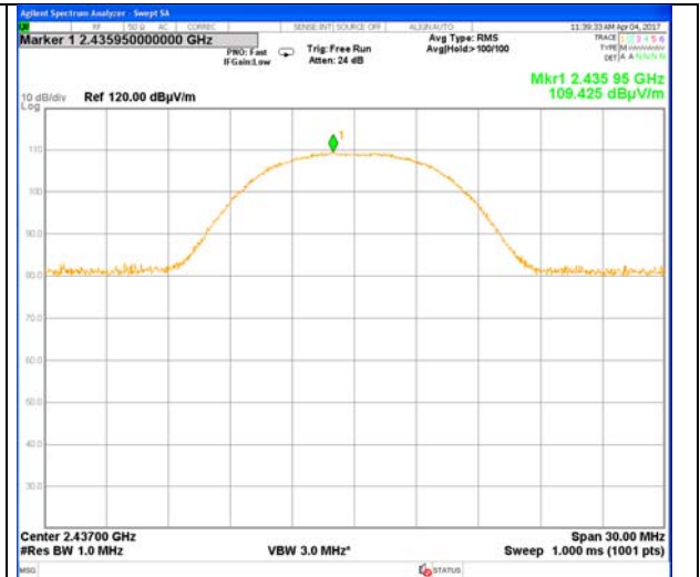
Plot # 14. Carrier frequency – 2437 MHz
