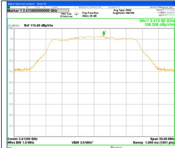
Plot # 16. Carrier frequency – 2412 MHz
