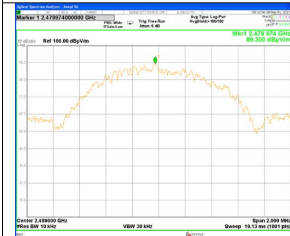
Plot # 36. Carrier frequency – 2480 MHz
