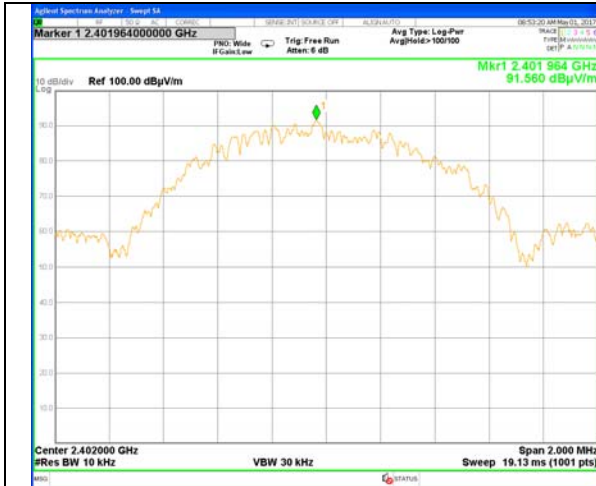
Plot # 34. Carrier frequency – 2402 MHz
