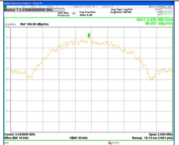
Plot # 35. Carrier frequency – 2440 MHz
