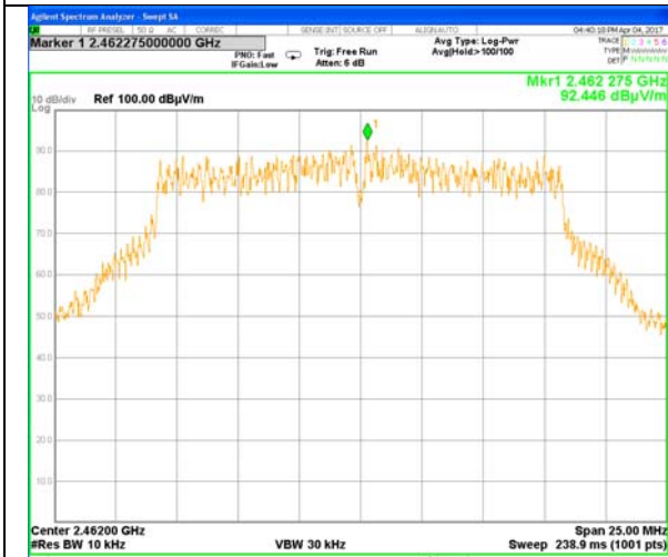
Plot # 30. Carrier frequency – 2462 MHz
