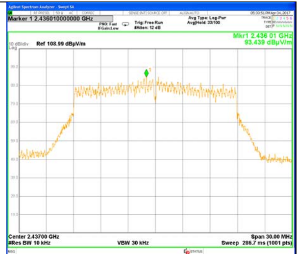
Plot # 32. Carrier frequency – 2437 MHz
