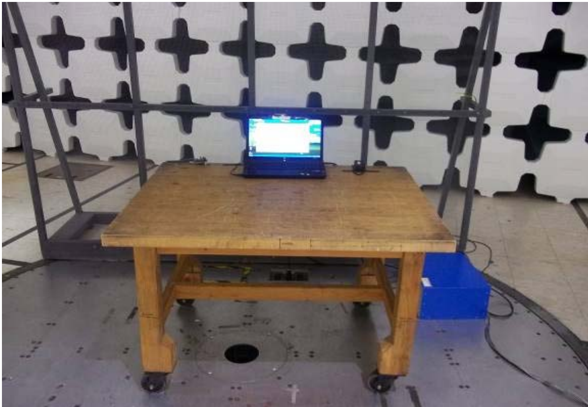
Test Configuration Photograph #1 (Conducted Emissions - Power Port)
