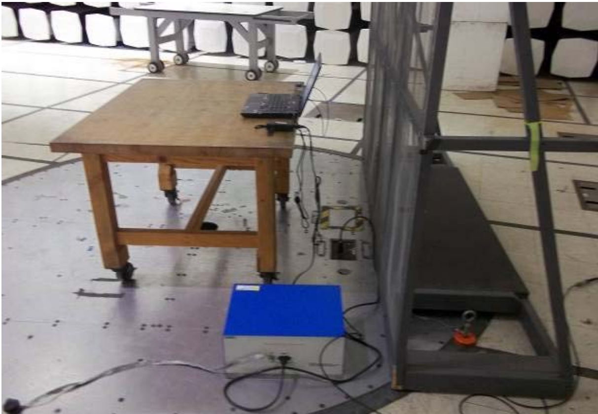
Test Configuration Photograph #2 (Conducted Emissions - Power Port)
