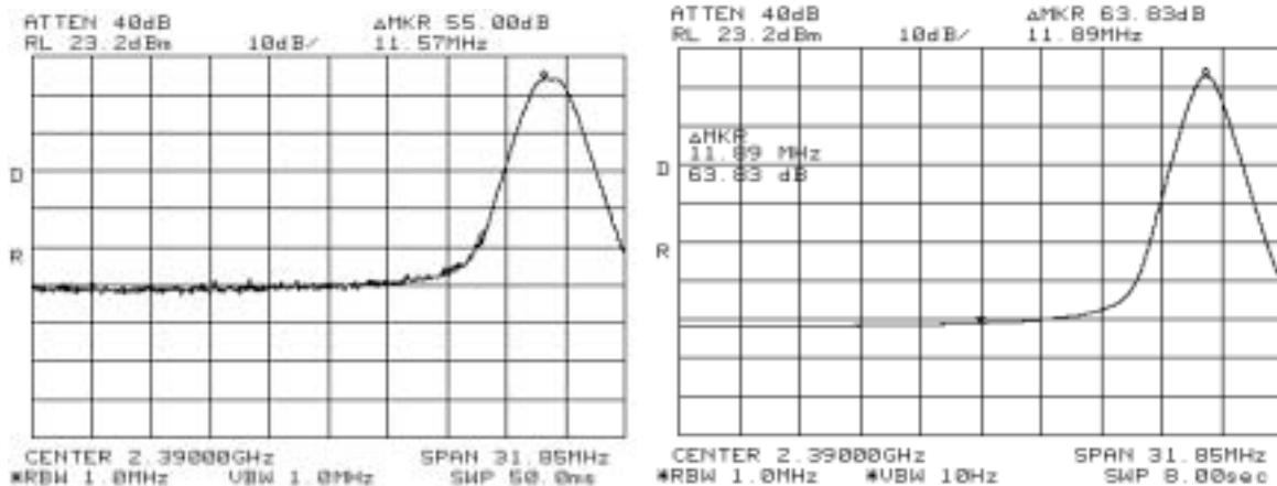
The highest signal level in the restricted bands above and below the allocated band was at the band edge. The highest peak and average field strengths in the restricted band are calculated from the field strength of the fundamental by subtracting a correction factor. The typical factor is the difference between the highest peak and average in band signal level and the highest peak and average restricted band levels.
