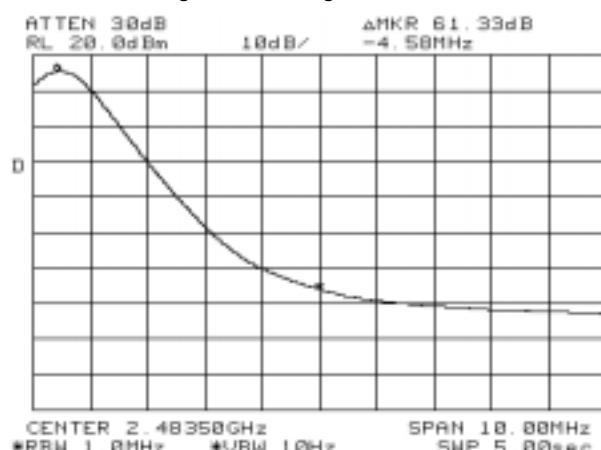
The highest signal level in the restricted bands above and below the allocated band was at the band edge. The highest peak and average field strengths in the restricted band are calculated from the field strength of the fundamental by subtracting a correction factor. The typical factor is the difference between the highest peak and average in band signal level and the highest peak and average restricted band levels.
