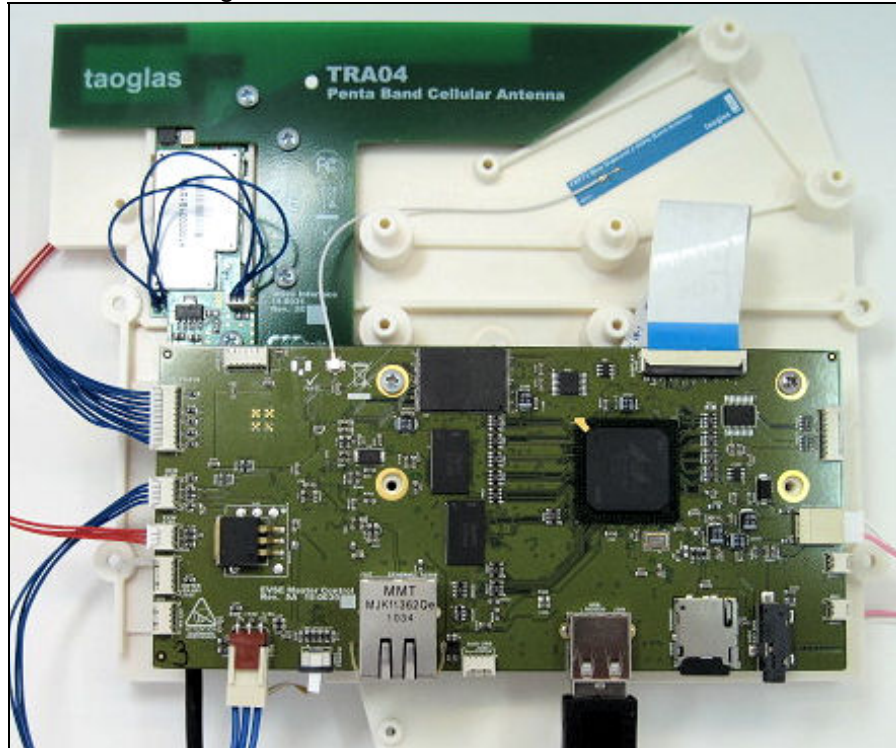
Unigen Module Mounted with New Antenna
