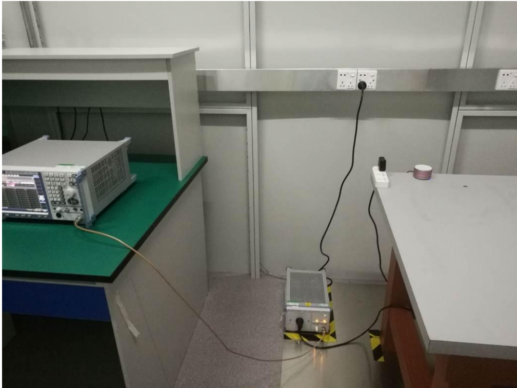
FCC RADIATED EMISSION TEST SETUP
