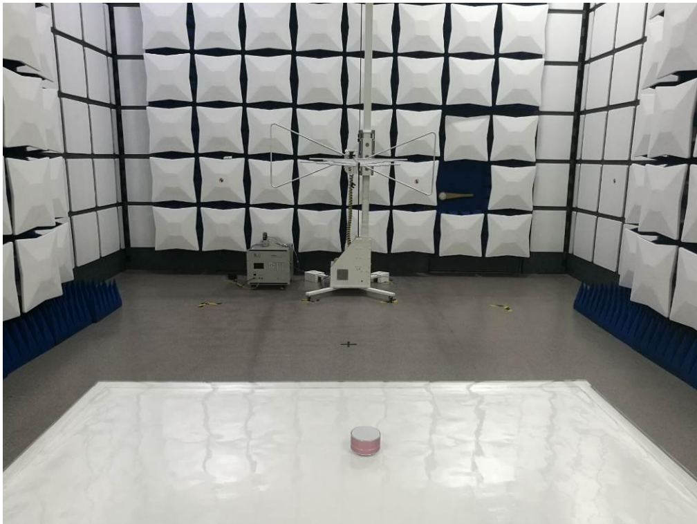
FCC RADIATED EMISSION TEST SETUP
