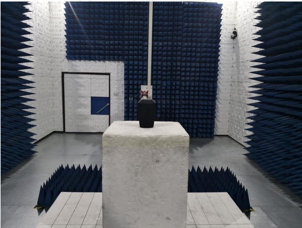
RADIATED EMISSION TEST SETUP ABOVE 1GHZ
