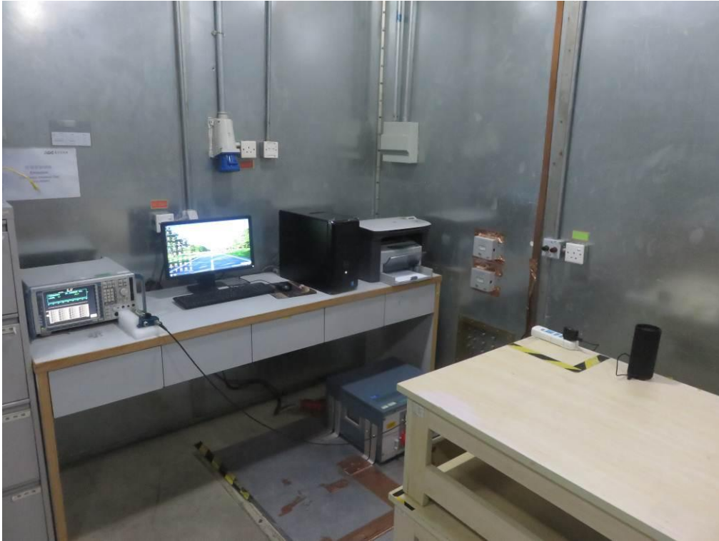
FCC RADIATED EMISSION TEST SETUP
