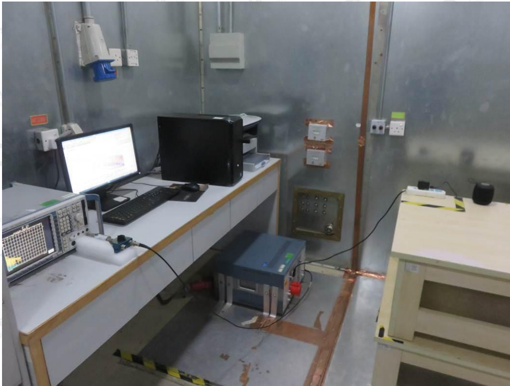
FCC RADIATED EMISSION TEST SETUP
