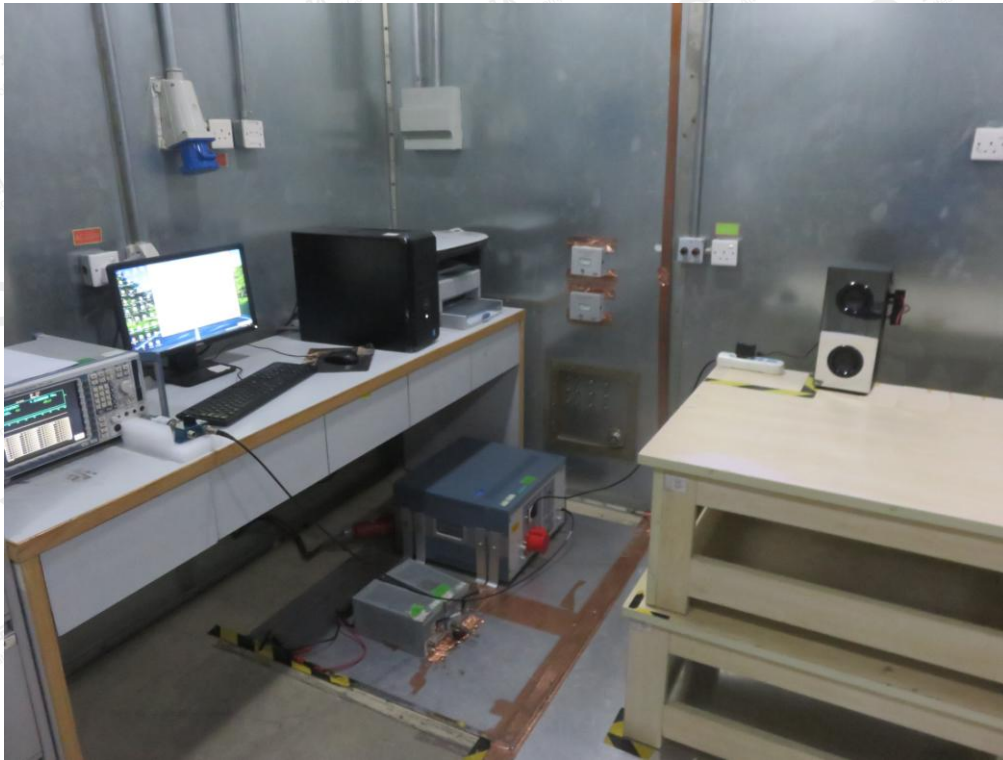
FCC RADIATED EMISSION TEST SETUP
