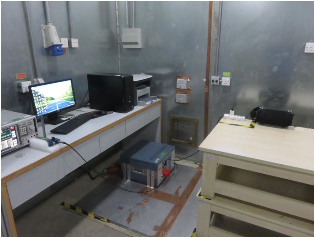
FCC RADIATED EMISSION TEST SETUP
