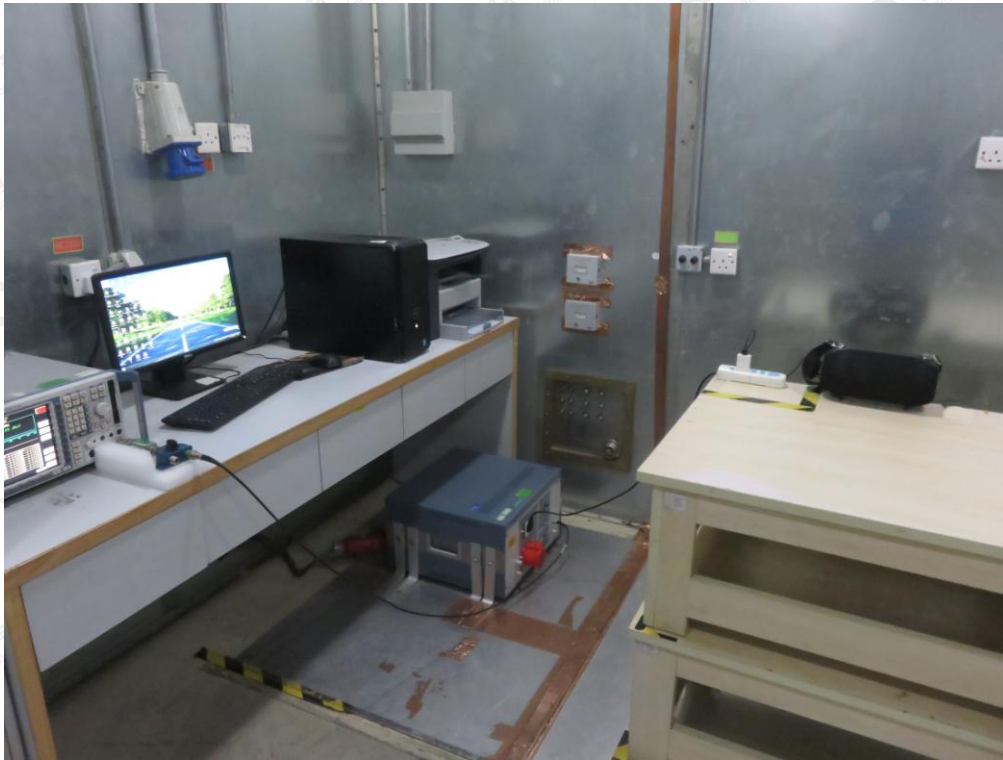
FCC RADIATED EMISSION TEST SETUP
