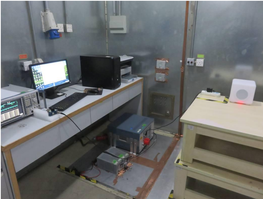
FCC RADIATED EMISSION TEST SETUP
