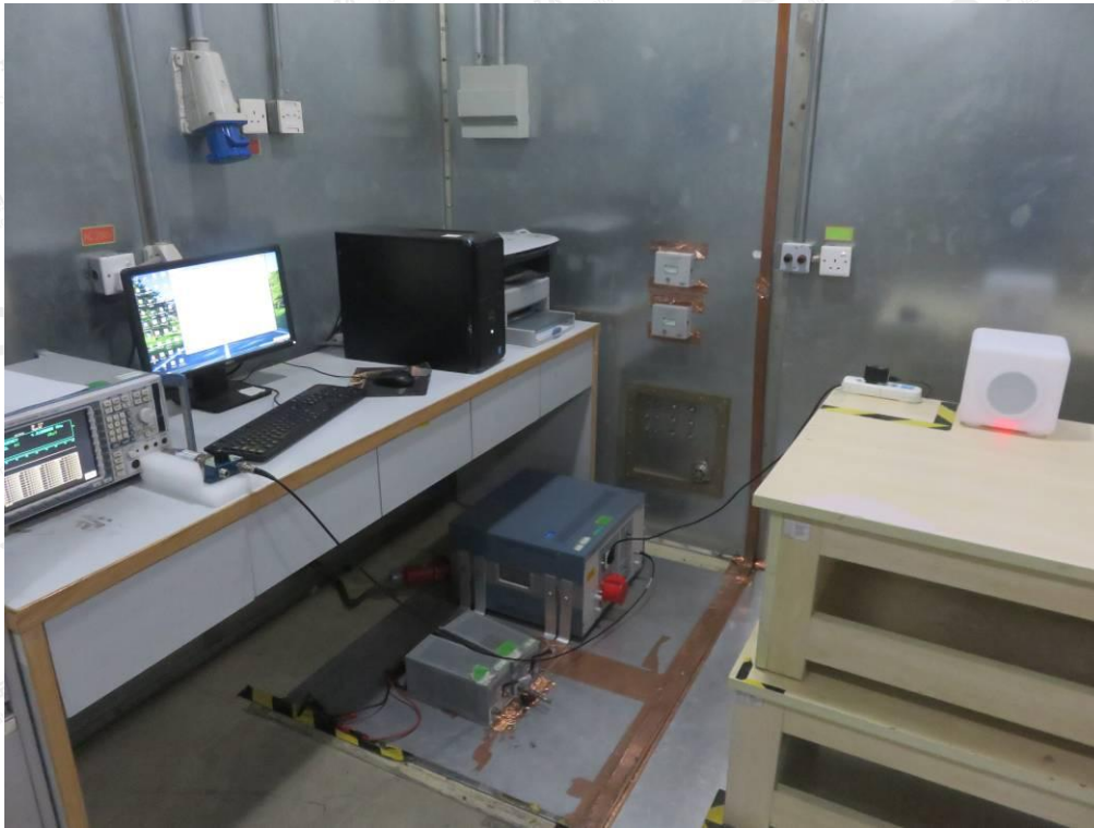
FCC RADIATED EMISSION TEST SETUP
