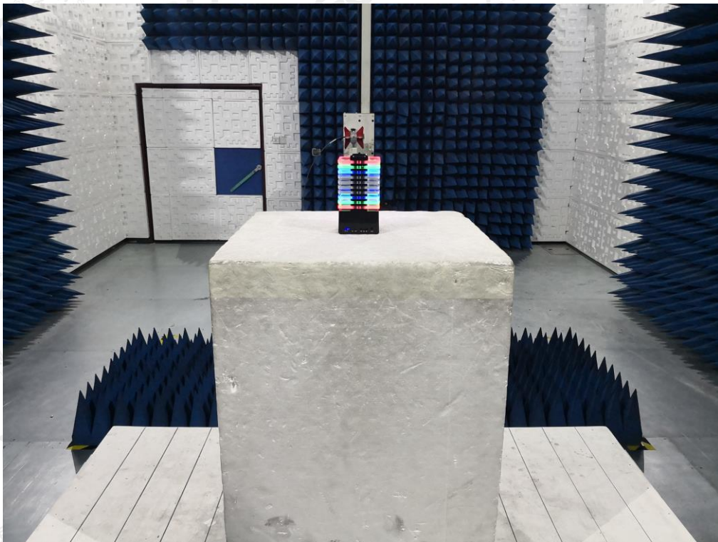
RADIATED EMISSION TEST SETUP ABOVE 1GHZ
