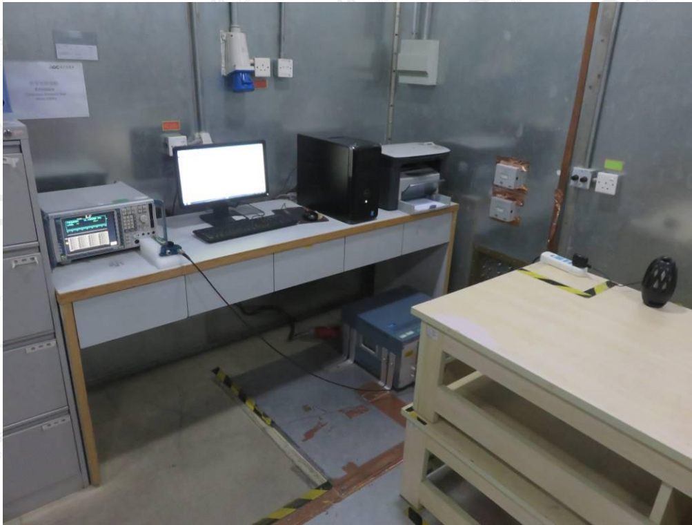
FCC RADIATED EMISSION TEST SETUP
