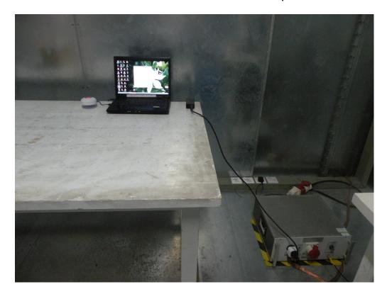
Radiated Emission Test Setup in Chamber
