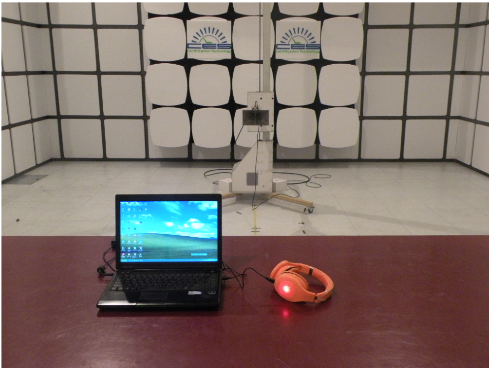
Radiated Emission Test Setup in Chamber
