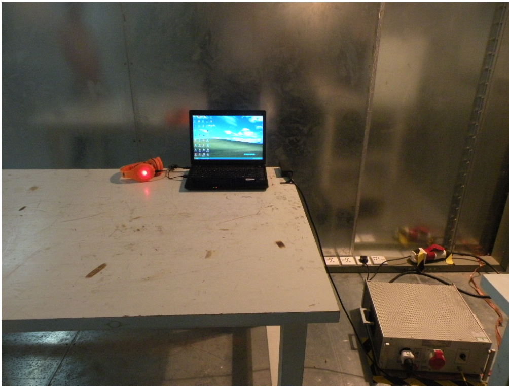
Radiated Emission Test Setup in Chamber
