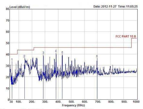
Condition : FCC PART 15 B POL: VERTICAL 3m
