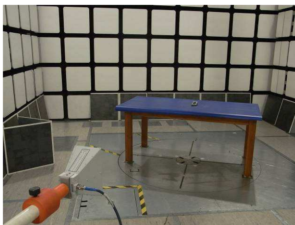
Set up for Radiated emission test
