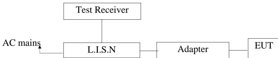
(EUT: HJ-Wireless Freezer Temperature Arrangement System-Centralized Controller)
