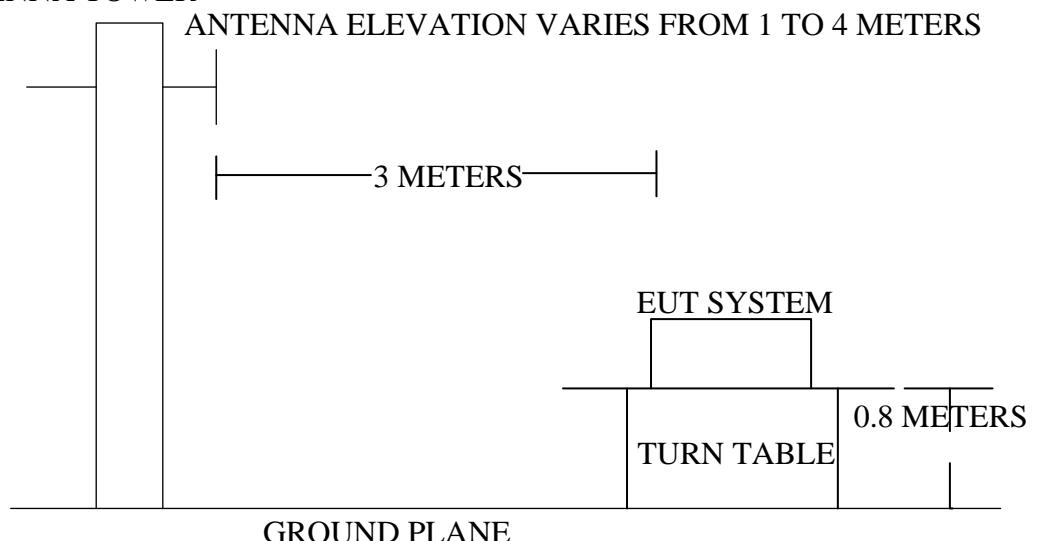
(EUT: HJ-Wireless Freezer Temperature Arrangement System-Centralized Controller)
