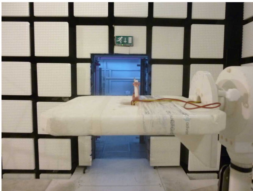
Photo 4: EUT at the anechoic chamber, stand-alone module with integrated antenna
