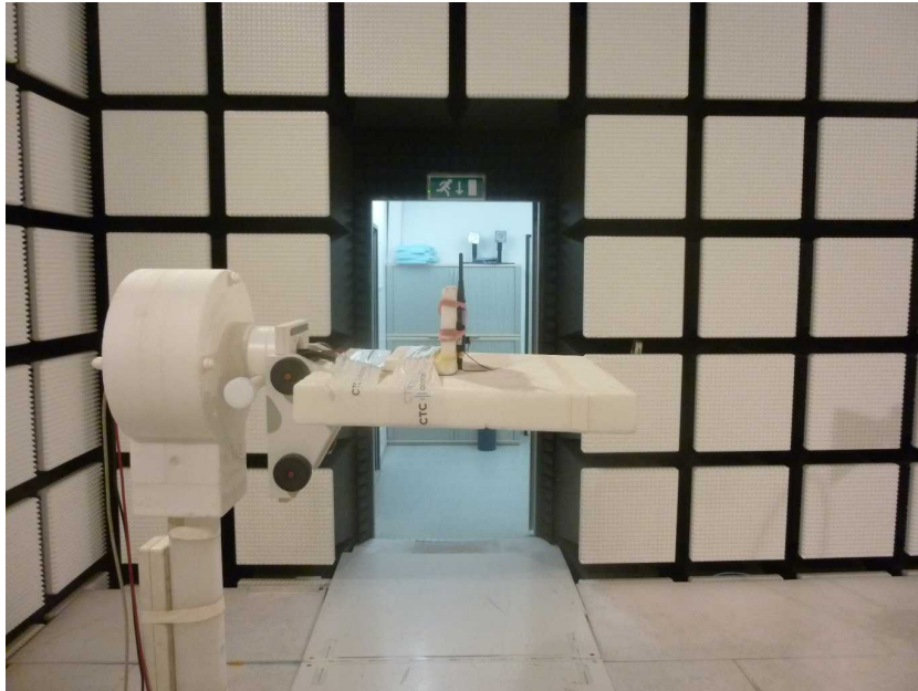
Photo 11: EUT at the anechoic chamber, module with external antenna
