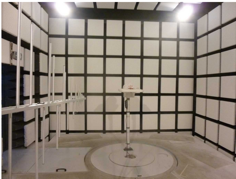
Photo 6: EUT at the anechoic chamber, stand-alone module with integrated antenna
