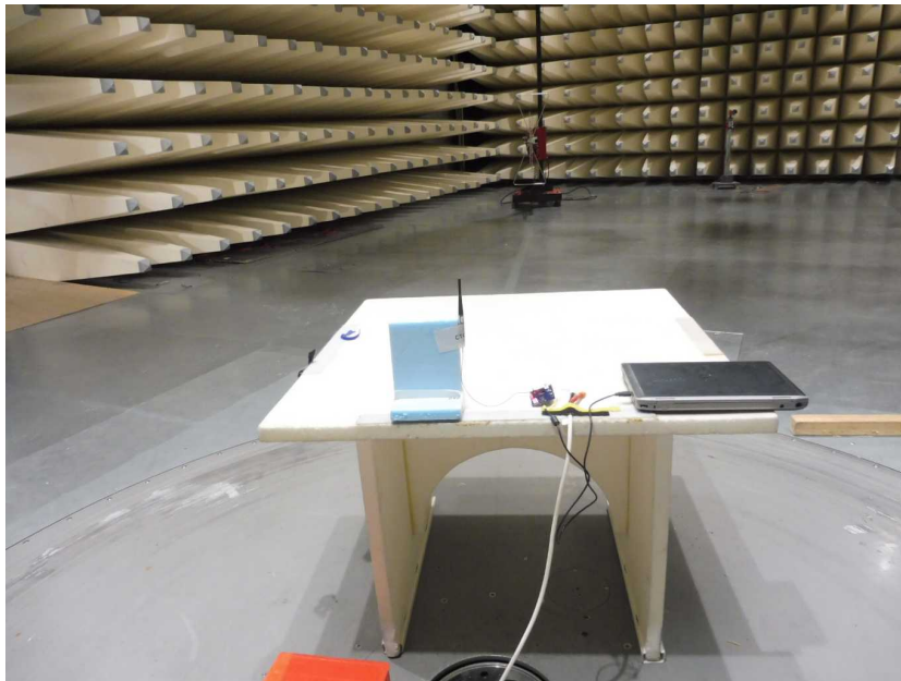
Photo 17: EUT at the semi-anechoic chamber, module with external antenna
