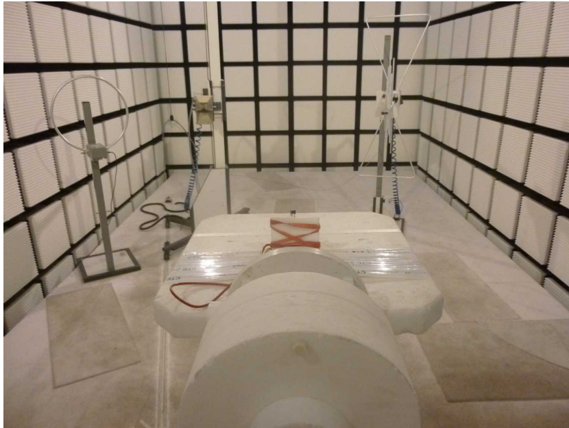
Photo 3: EUT at the anechoic chamber, stand-alone module with integrated antenna
