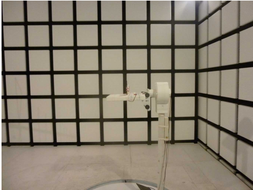
Photo 9: EUT at the anechoic chamber, module with external antenna
