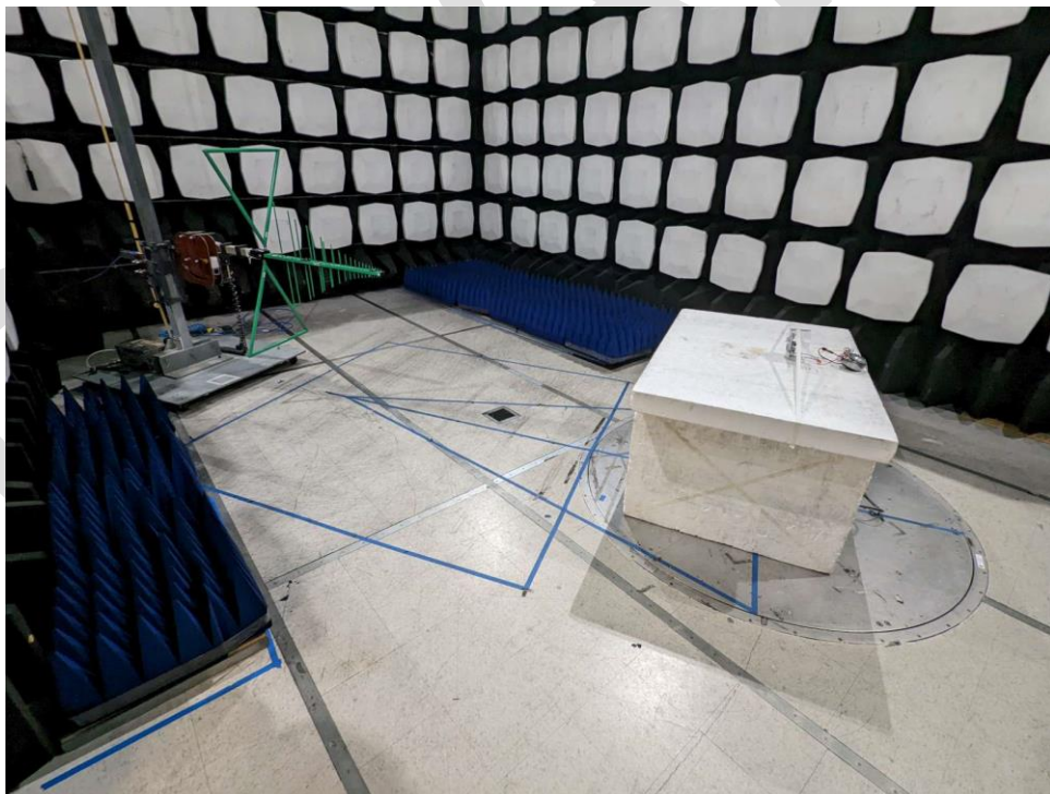
Figure2 – Test Set up - Radiated Emissions <1 GHz
