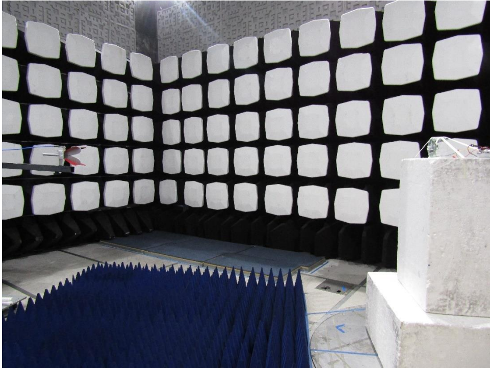
Figure3 – Test Set up - Radiated Emissions <10 GHz
