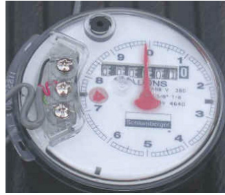
Figure 2.7 Threading the cable around the strain relief posts
