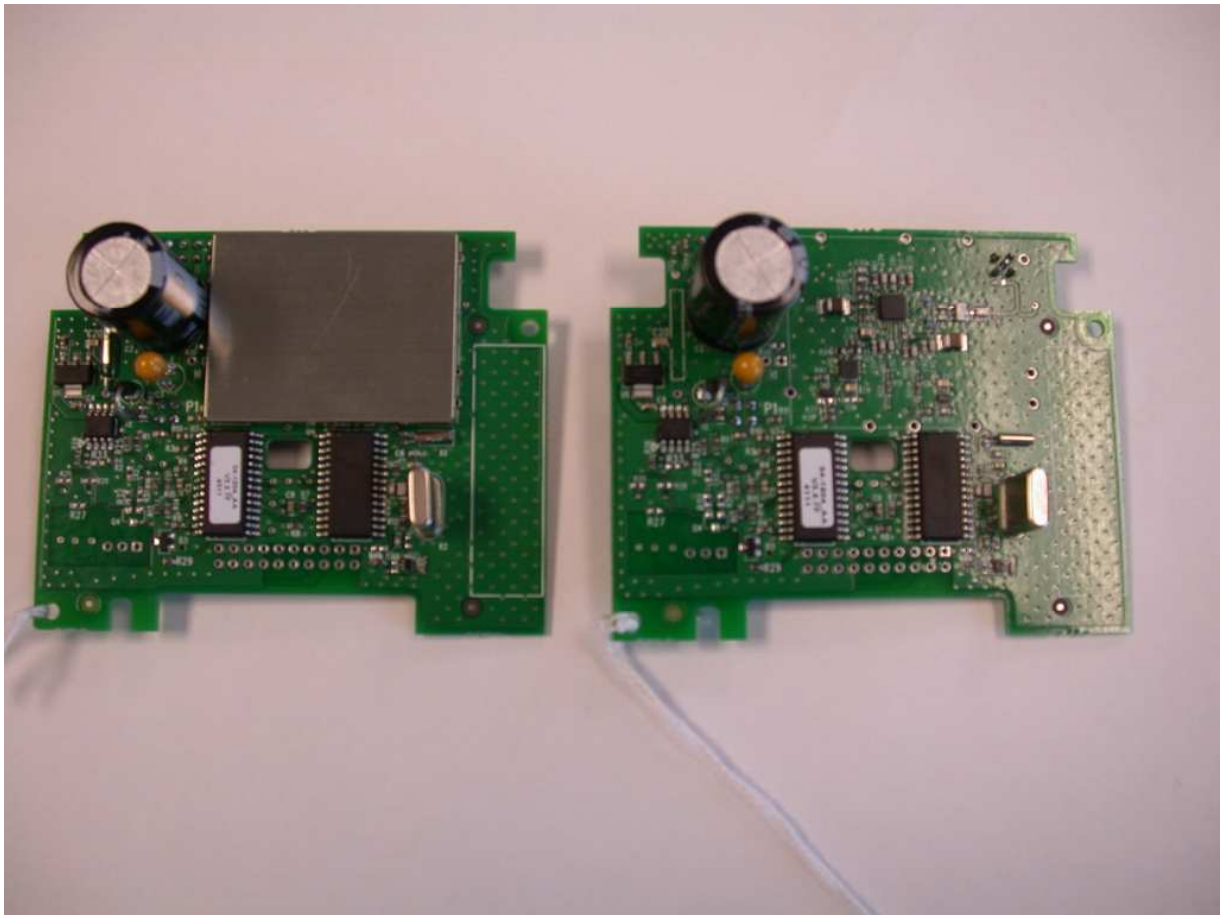
Figure 1: Internal Photo – With and Without Shield
