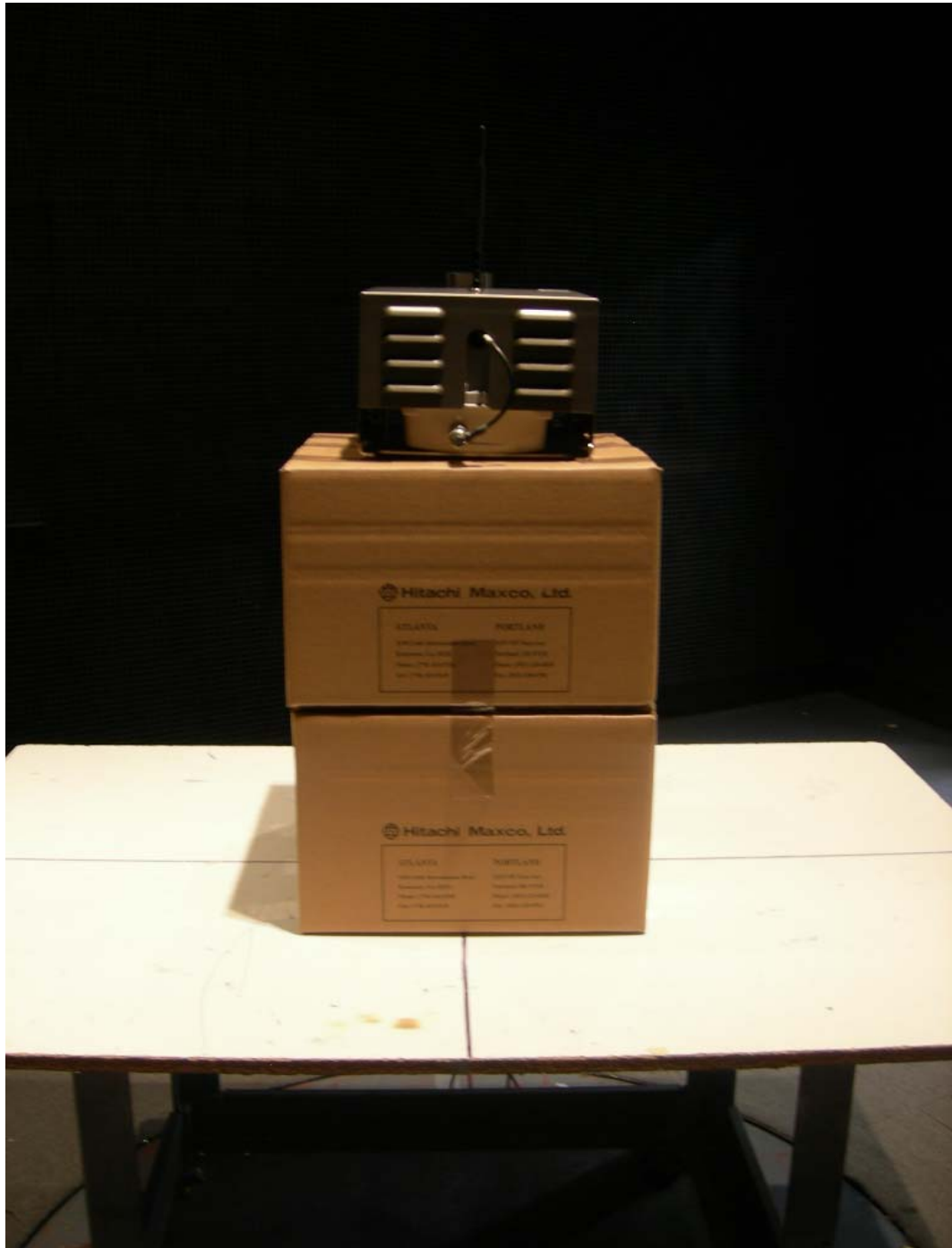
Figure 1: Radiated Emissions (Pole Mount Hardware)
