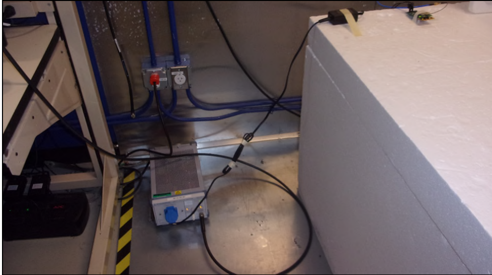
Figure 8: Equipment Under Test – AC Conducted Emissions
