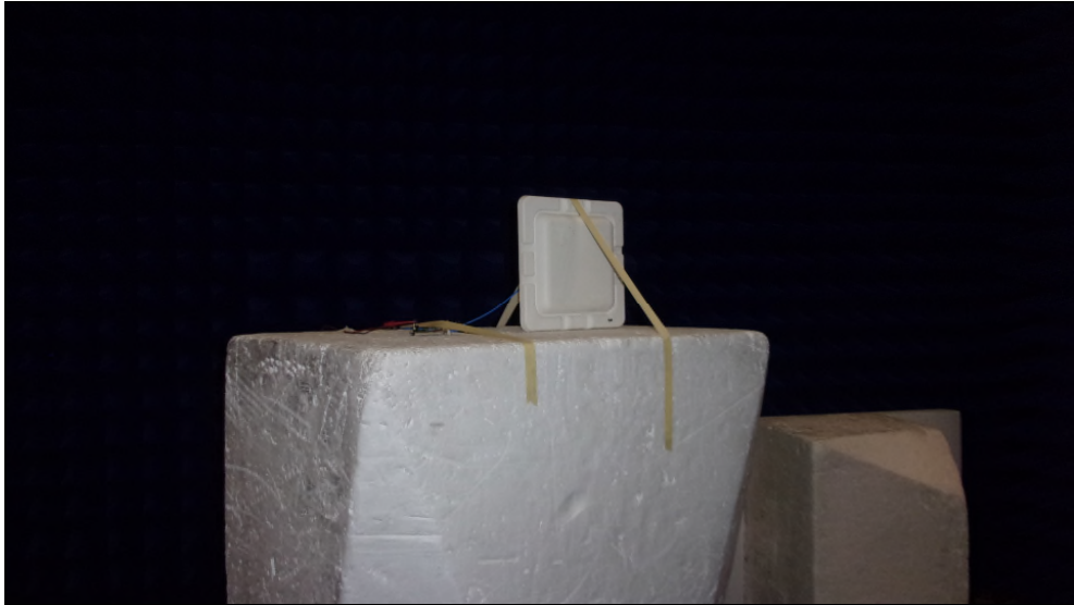
Figure 5: Equipment Under Test – Radiated Emissions >1GHz
