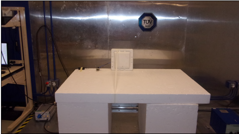
Figure 7: Equipment Under Test – AC Conducted Emissions
