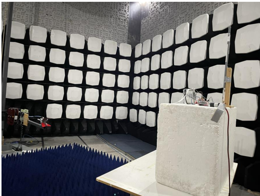
Figure:6– Test Set up – Rear View of the EUT - Radiated Emissions <10 GHz
