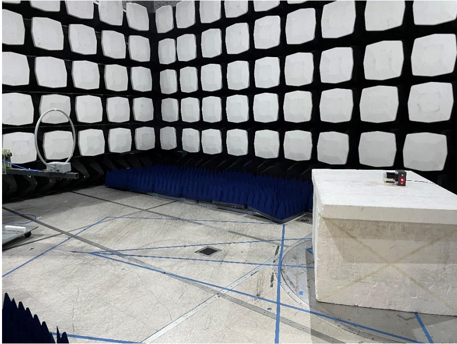
Figure:1 – Test Set up - Radiated Emissions <30 MHz
