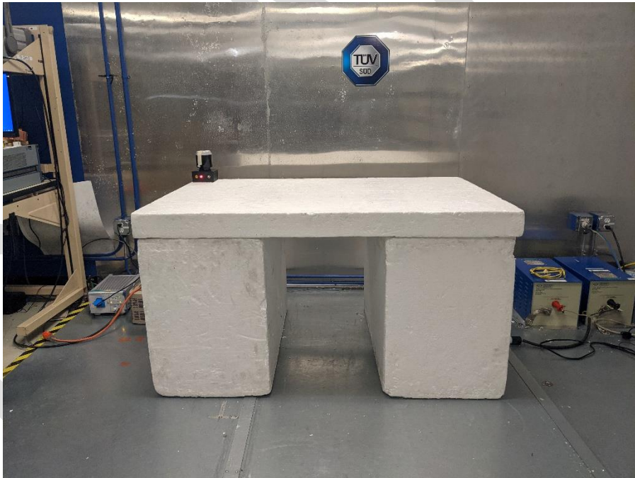
Figure:4 – Test Set up – Conducted Emissions
