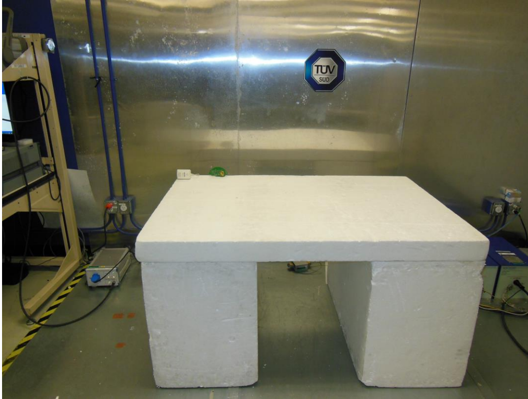
Figure 7: Equipment Under Test – AC Conducted Emissions
