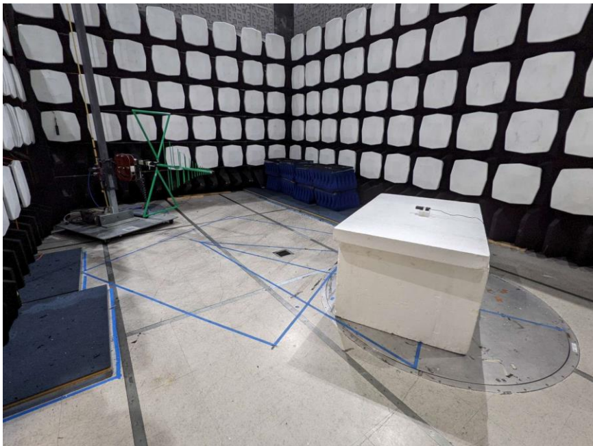
Figure A-2 – Test Set up - Radiated Emissions <1 GHz
