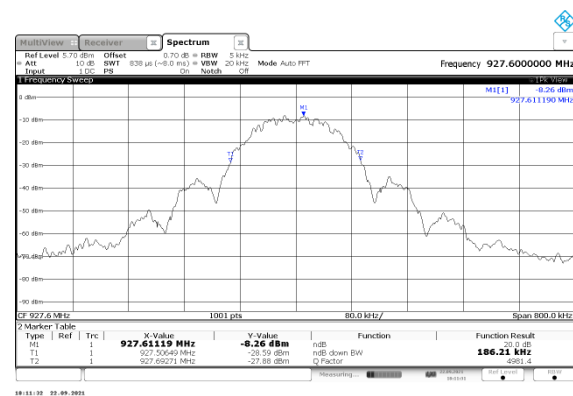
Figure 2.3.6-8: 20dB BW High Channel – 150 kbps
