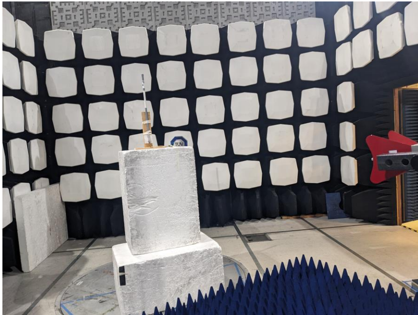
Figure5 – Front View Test Set up - Radiated Emissions <10 GHz
