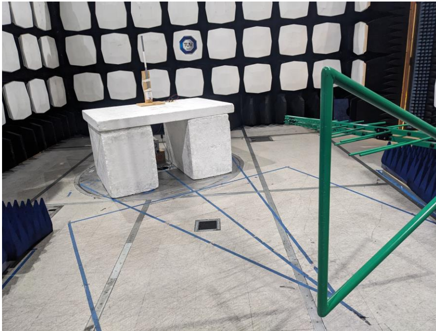
Figure3 – Front View Test Set up - Radiated Emissions <1 GHz
