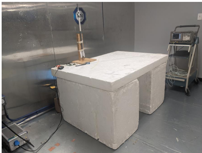
Figure8 – Side View Test Set up –AC Power Line Conducted Emissions
