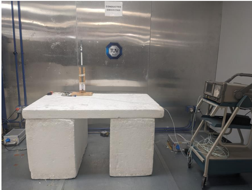
Figure7 – Front View Test Set up – AC Power Line Conducted Emissions
