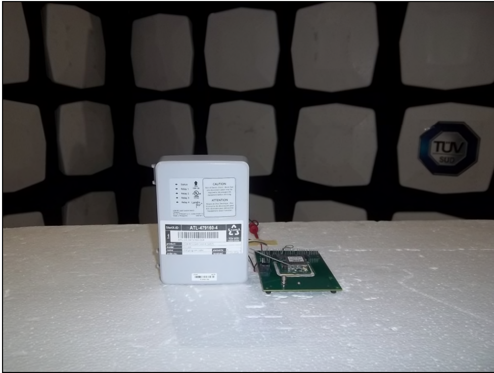
Figure 3: Equipment Under Test – Radiated Emissions – Z-orientation
