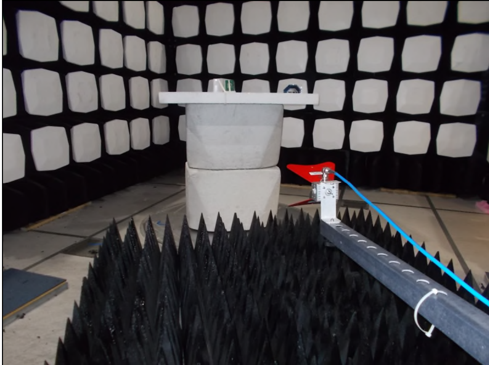
Figure 8: Equipment Under Test – Radiated Emissions – 1GHz - 10GHz
