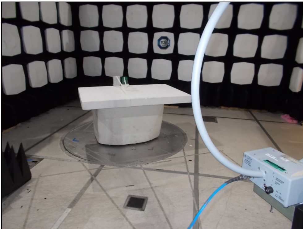
Figure 4: Equipment Under Test – Radiated Emissions – 9kHz - 30MHz
