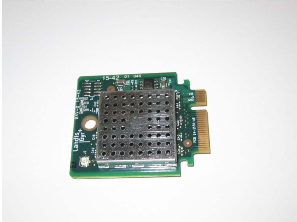
Figure 1 - 3. Gridstream Series 5 Single Board Radio Rear View, I/O Connector, Pin 1 (Red Arrow)
