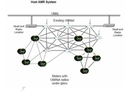
Data acquisition can be provided by a hosted service for small to large meter deployments or an own and operate solution. The UtiliNet network provides secure, packet based data transfer. UtiliNet PCMCIA IWR Card supports the following system services:
