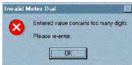
Figure 7 - 20. Error Message Displayed when Entered Read is too large for the Rollover Point
