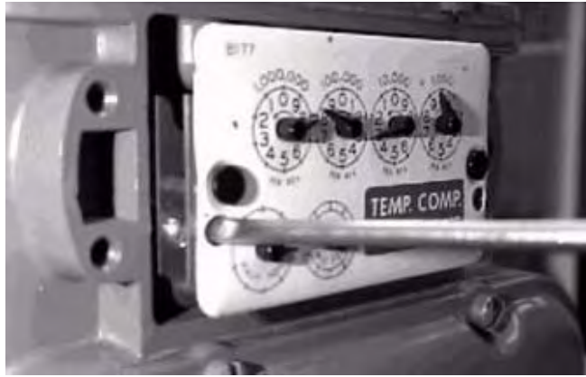
Figure 6 - 4. Removing the Index (one screw on each side)
