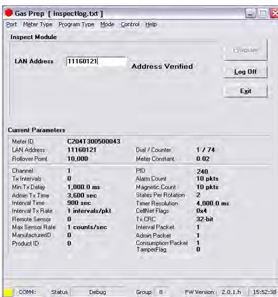
Figure 7 - 10. "Inspect Mode" With Power LAN Scanned In
