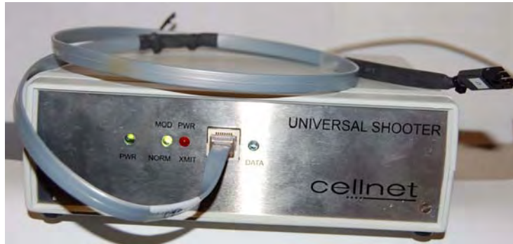
Figure 7 - 2. Shooter box with data cable
