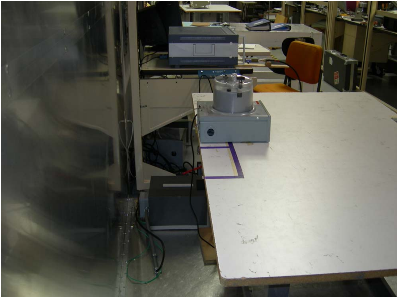
Figure 5: Test Set Up – Conducted Emissions
