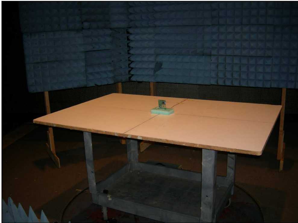
Figure 1: Test Setup Photo - Radiated Emissions
