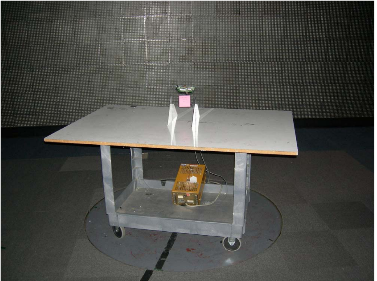
Figure 4: Test Setup - Radiated Emissions – Unintentional
