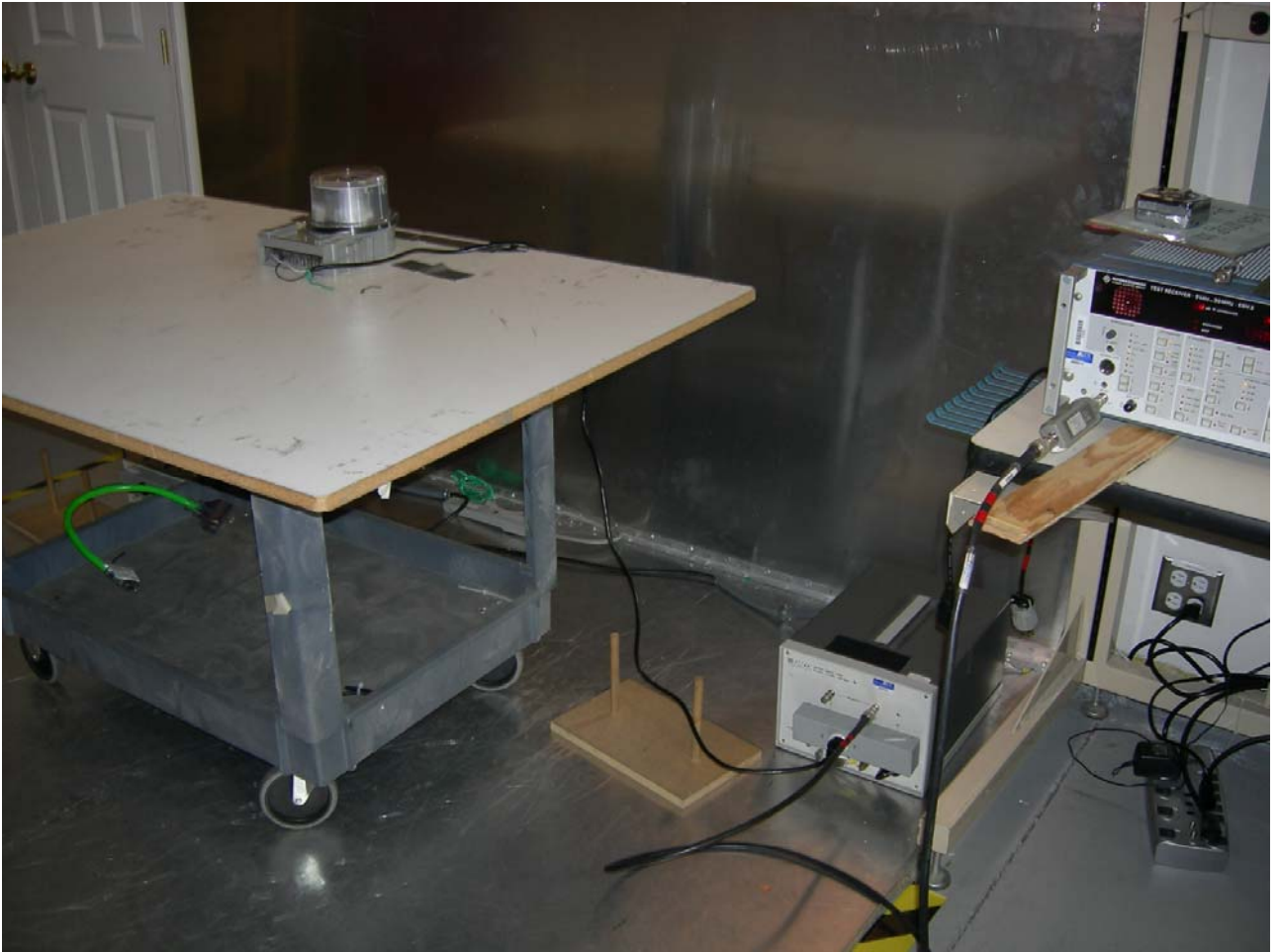
Figure 5: Test Setup - Conducted Emissions
