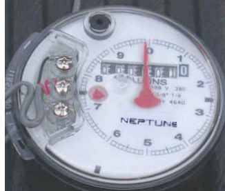
Figure 2 - 3. Threading the cable around the strain relief posts
