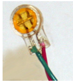
Figure A - 1. Stripped wires pushed into Scotchlok connector
