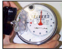
Figure 2 - 4. Applying moisture compound
