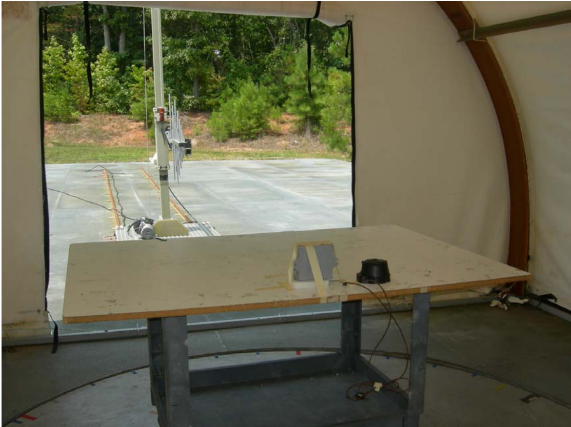
Figure 1: Test Setup - Radiated Emissions
