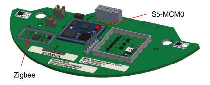
Figure 1. I210+c module, top side with shield lids removed
