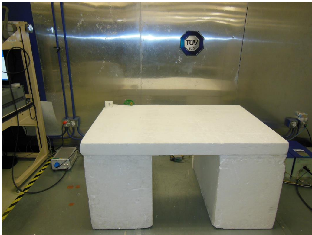
Figure 8: Equipment Under Test – AC Conducted Emissions
