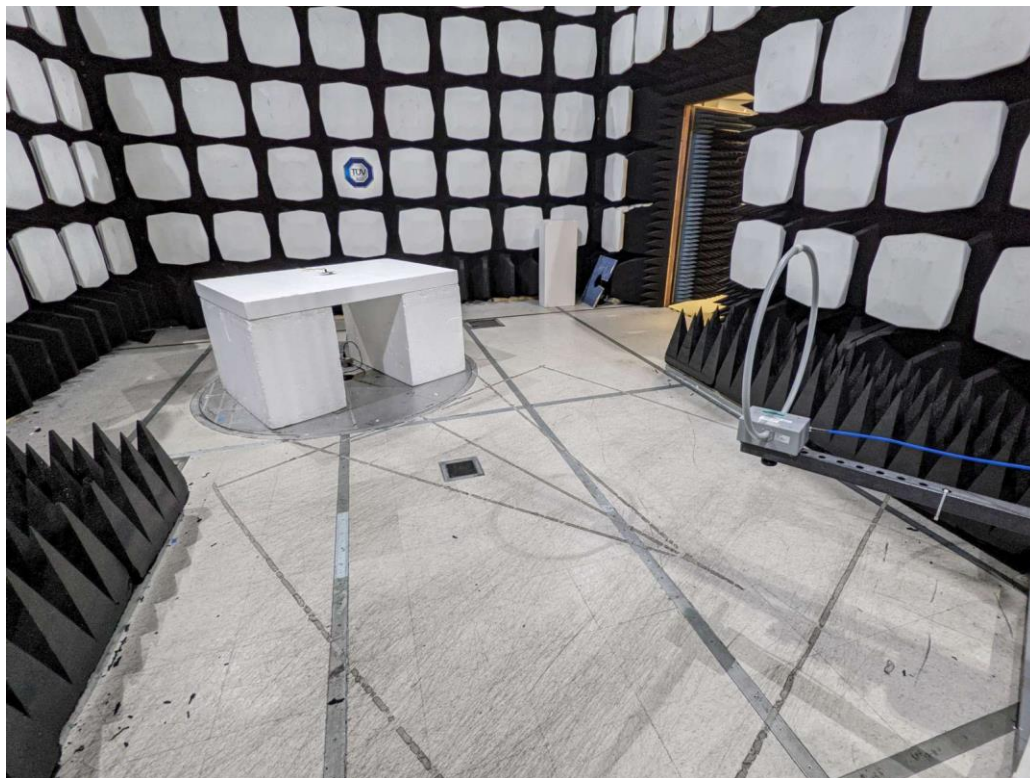
Figure 2: Equipment Under Test – Radiated Emissions <30MHz
