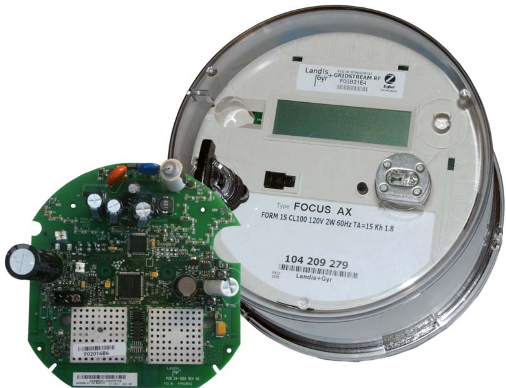
Figure 1. Gridstream RF Enhanced Integrated FOCUS AX module and the Landis+Gyr FOCUS AX meter
