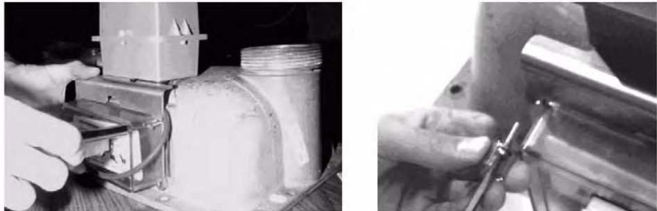
Figure 6.23 Sprague/Actaris: installing Index cover
