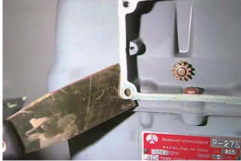
Figure 5.16 Rockwell/Equimeter/Sensus: Removal of index cover gasket
