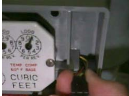
Figure 5.19 Rockwell/Equimeter/Sensus: Connecting the battery
