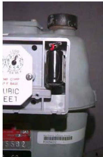
Figure 5.20 Rockwell/Equimeter/Sensus: Correct battery orientation (connector on top)
