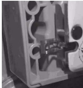
Figure 5.7 American: Installing Index on standoff screws
