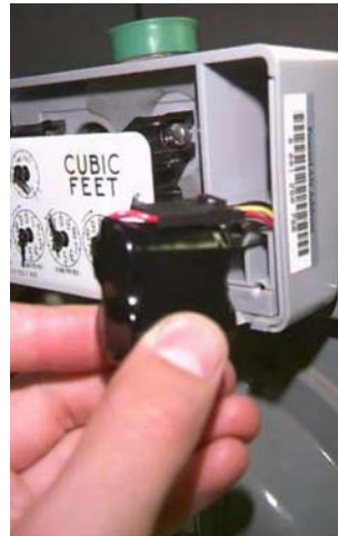
Figure 5.50 Lancaster/National: Correct Battery Orientation
