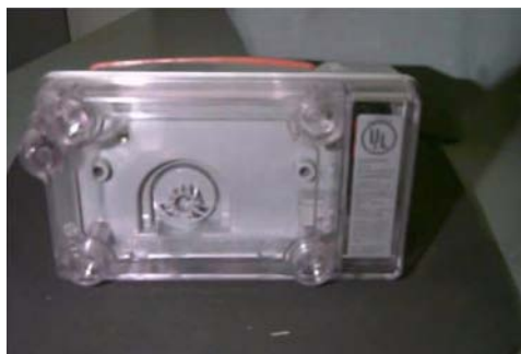
Figure 5.13 Rockwell/Equimeter/Sensus: meter module before installation
