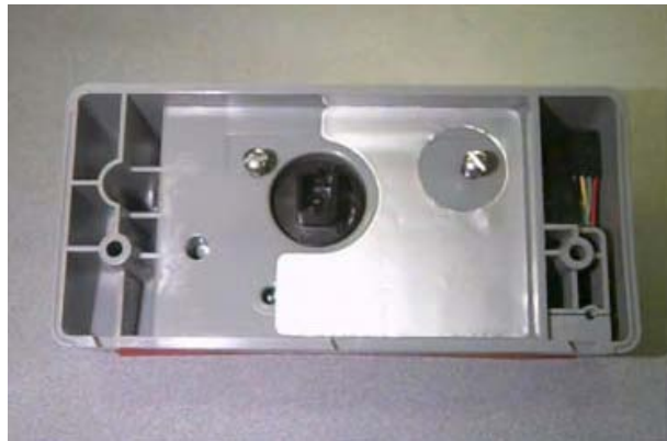
Figure 5.46 Lancaster/National: Meter Module pre-assembled
