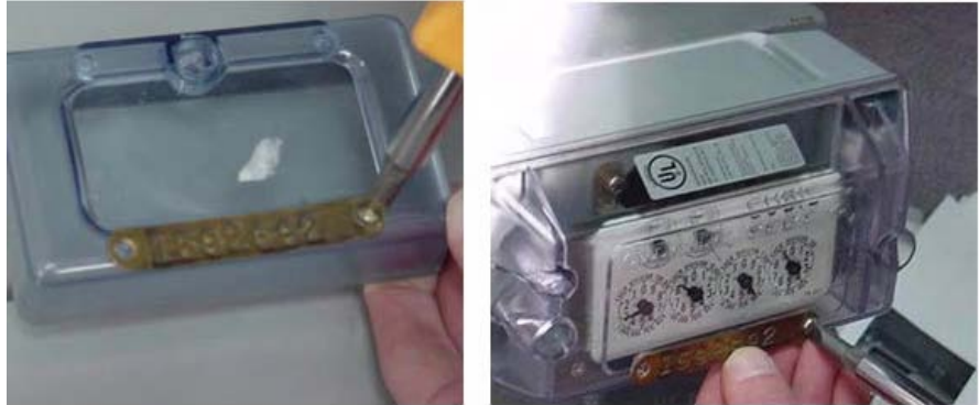
Figure 5.53 Lancaster/National: Replacing Serial Number Plate
