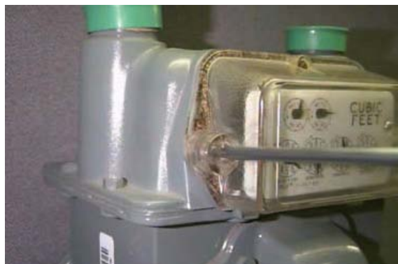
Figure 5.27 Sprague/Schlumberger/Actaris: Removing the index cover
