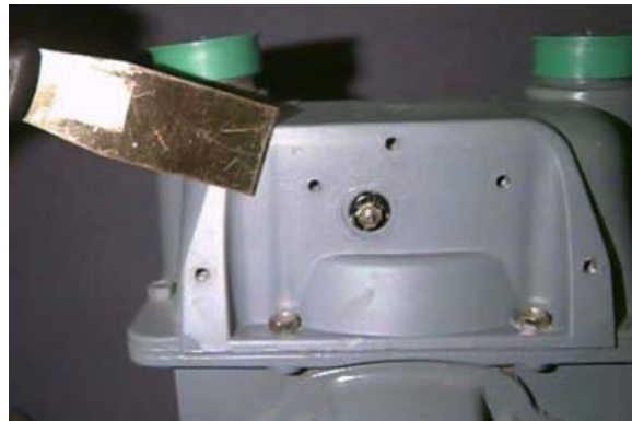
Figure 5.29 Sprague/Schlumberger/Actaris: Removal of index cover gasket
