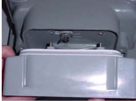
Figure 5.47 Lancaster/National: Alignment of the meter drive dog and screws
