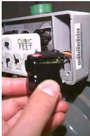
Figure 5.35 Sprague/Schlumberger/Actaris: Correct Battery Orientation
