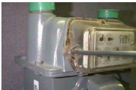
Figure 5.27 Sprague/Schlumberger/Actaris: Removing the index cover
