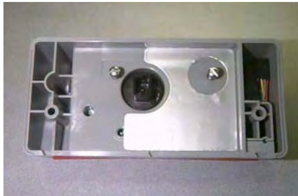
Figure 5.46 Lancaster/National: Meter Module pre-assembled
