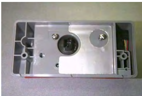
Figure 5.25 Sprague/Schlumberger/Actaris: Meter Module before installation
