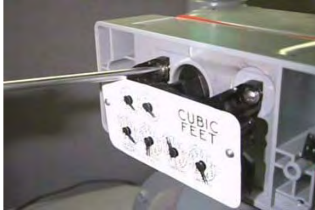
Figure 5.33 Sprague/Schlumberger/Actaris: Securing index and checking for free movement of wiggler-
