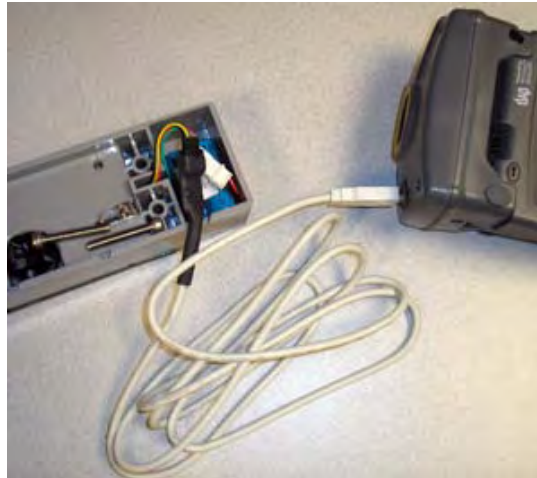
Figure 6.8 American CG3:Connecting the programming cable to the American Commercial meter module
