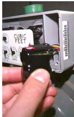
Figure 5.50 Lancaster/National: Correct Battery Orientation
