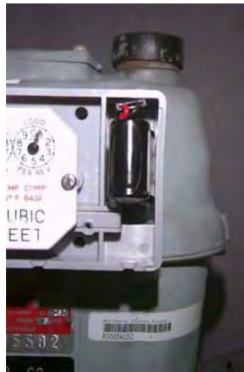
Figure 5.20 Rockwell/Equimeter/Sensus: Correct battery orientation (connector on top)
