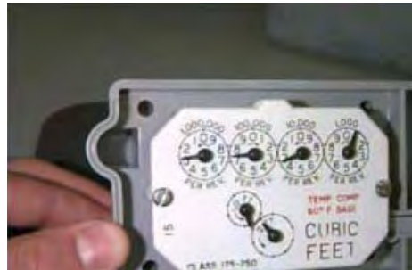
Figure 5.17 Rockwell/Equimeter/Sensus: Meter Module and index with screws in place ready for assembly
