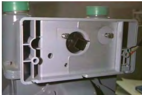
Figure 5.48 Lancaster/National: Meter Module base attached to meter, ready to slide on dials
