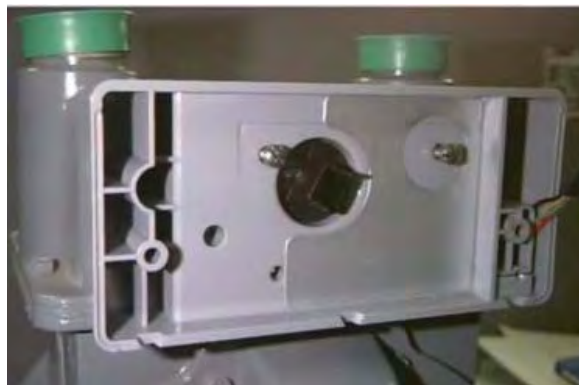
Figure 5.32 Sprague/Schlumberger/Actaris: Meter Module base attached to meter, ready to slide on dials
