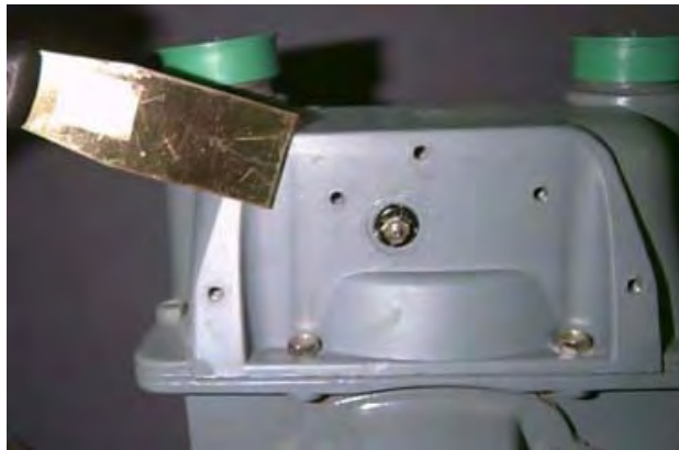
Figure 5.44 Lancaster/National: Removal of index cover gasket
