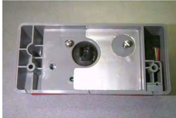
Figure 5.30 Sprague/Schlumberger/Actaris: Meter Module pre-assembled
