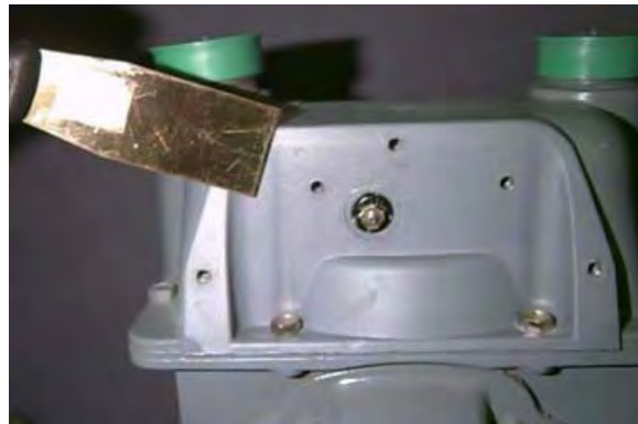
Figure 5.29 Sprague/Schlumberger/Actaris: Removal of index cover gasket
